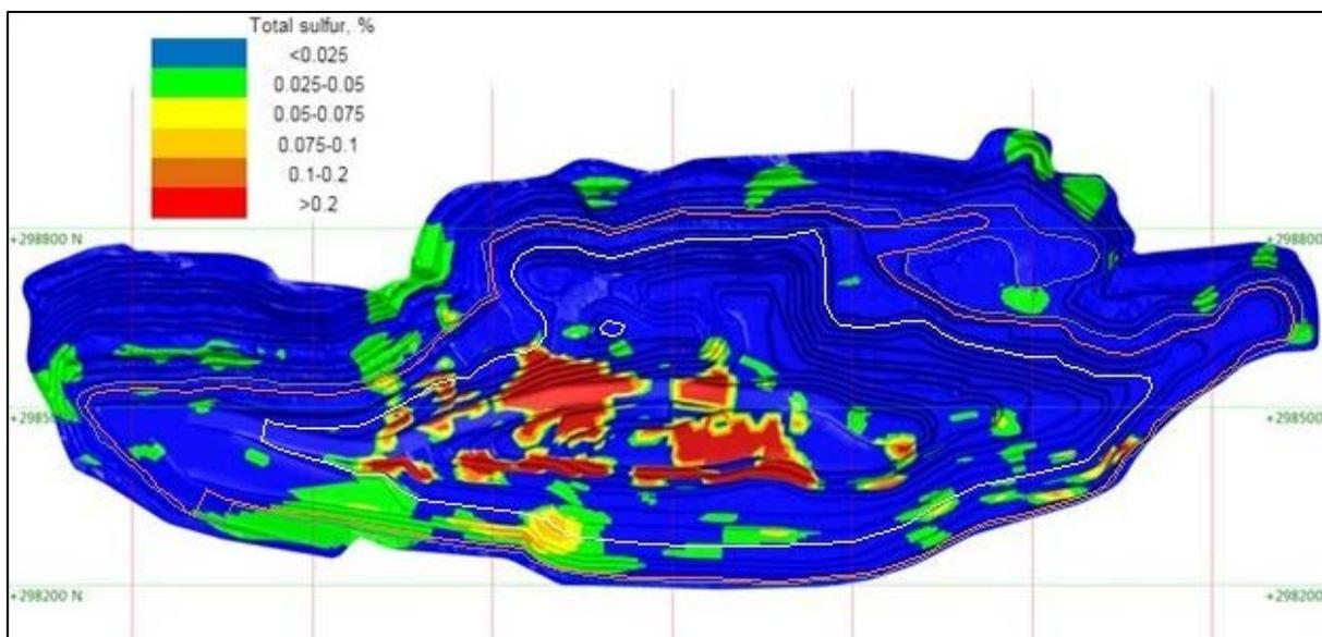
**Figure 7: Leapfrog image of the pit shell showing the distribution of sulfur on the pit walls**
