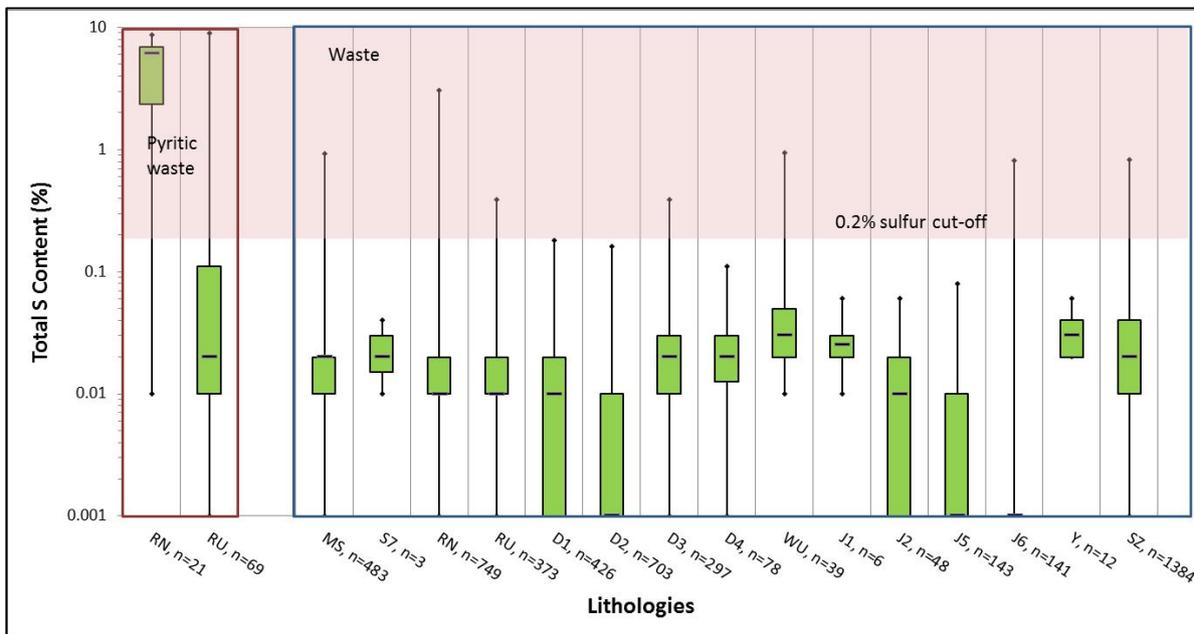
**Figure 3: Box and whisker plots showing sulfur statistics in waste materials, by lithology (Linklater et al., 2015)**
