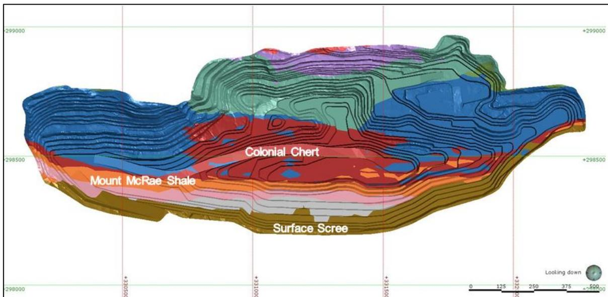
**Figure 6: Leapfrog image of the pit shell, and showing lithological composition of the pit walls**
