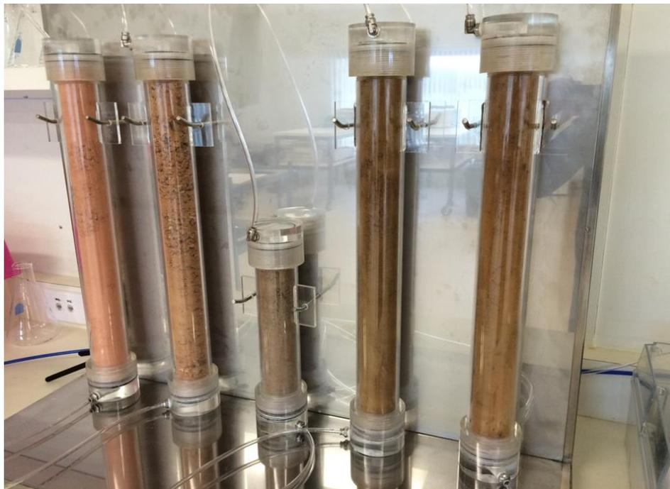
Figure 9. Saturated column setup
