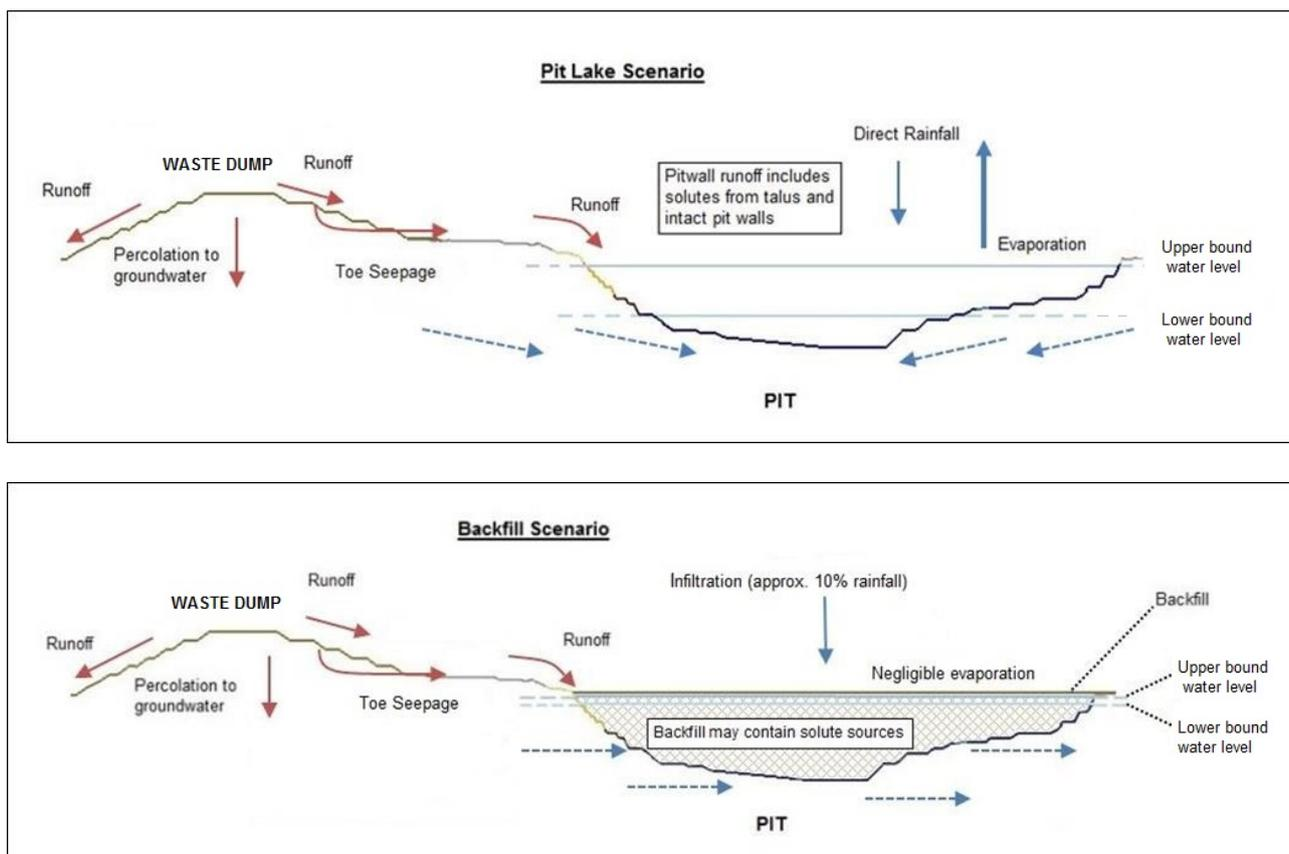
**Figure 8: Schematic representations of a pit void showing (i) pit lake formation and (ii) backfilled pit closure scenarios**
