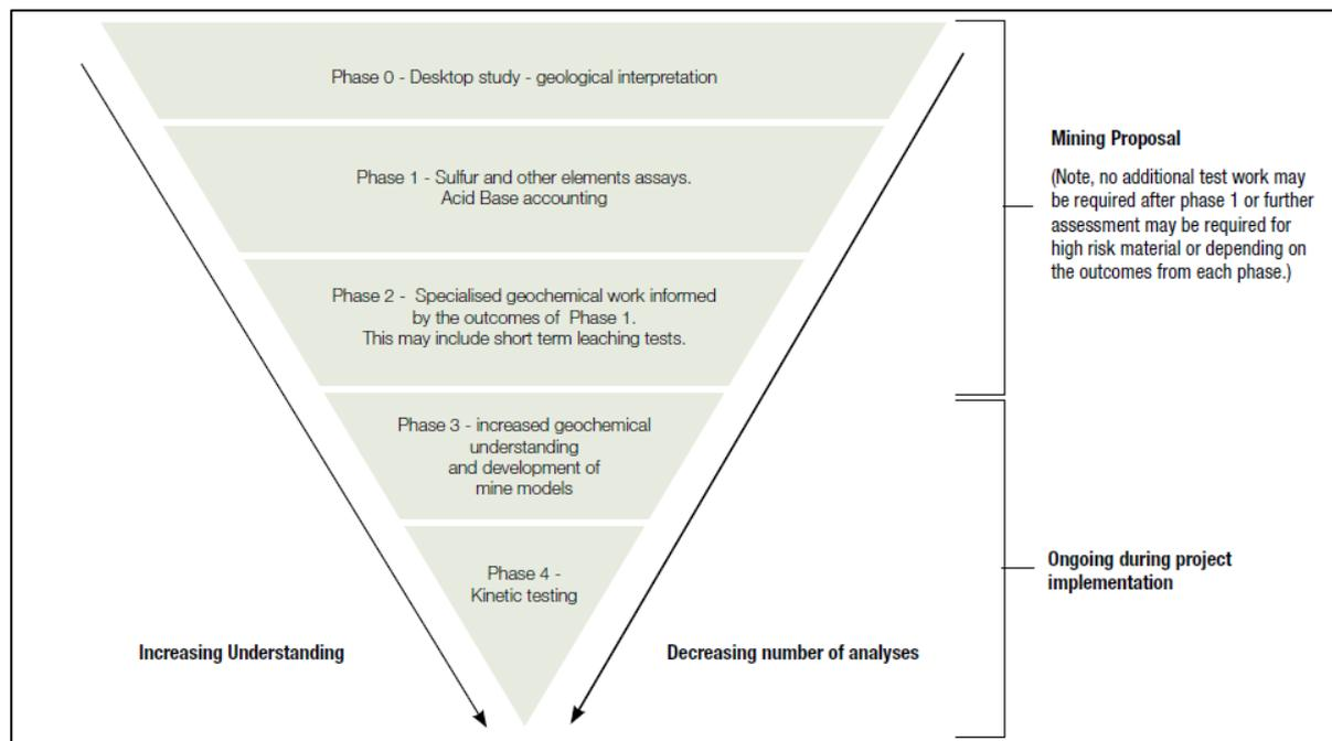
**Figure 1: Phases of geochemical materials characterisation (DMP, 2016)**
