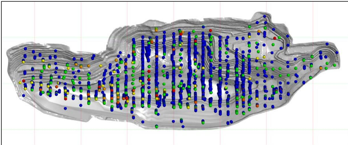
**Figure 4: Image of pit shell showing spatial distribution of drill holes with sulfur data**
