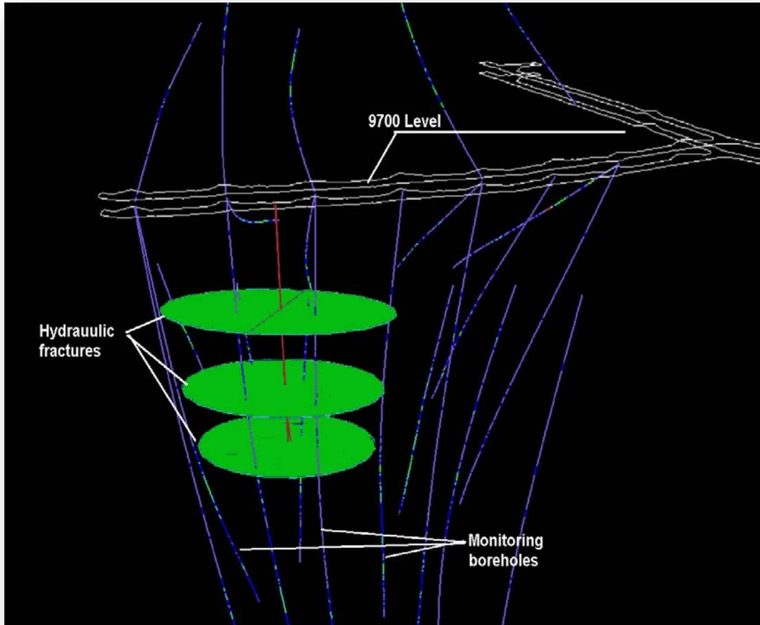
Transform a highly competent rock mass (primary rock) into a rock mass material appropriate for caving methods.
