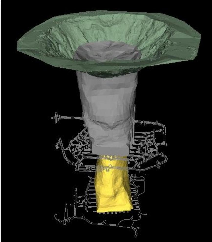
The risk of poor subsidence estimates is typically related to infrastructure location outside the subsidence limits (below). In smaller footprints and strong rock masses the subsidence angles could be negative (overhang) resulting in ore loss and early dilution!
