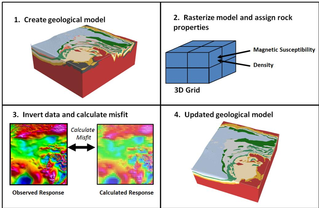
**Figure 3: Generalised workflow of the constrained inversion process**
