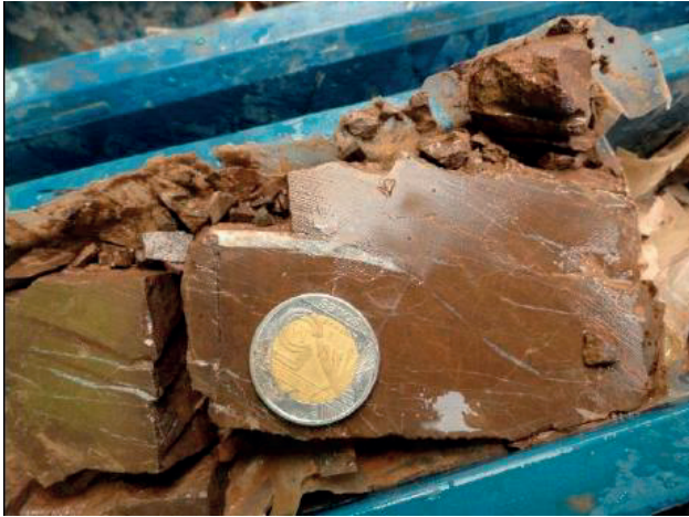
Figure 1. Rock with micro-defects (cemented with calcite) where induced breaks were generated by drilling. RQD assessment was underestimated.
