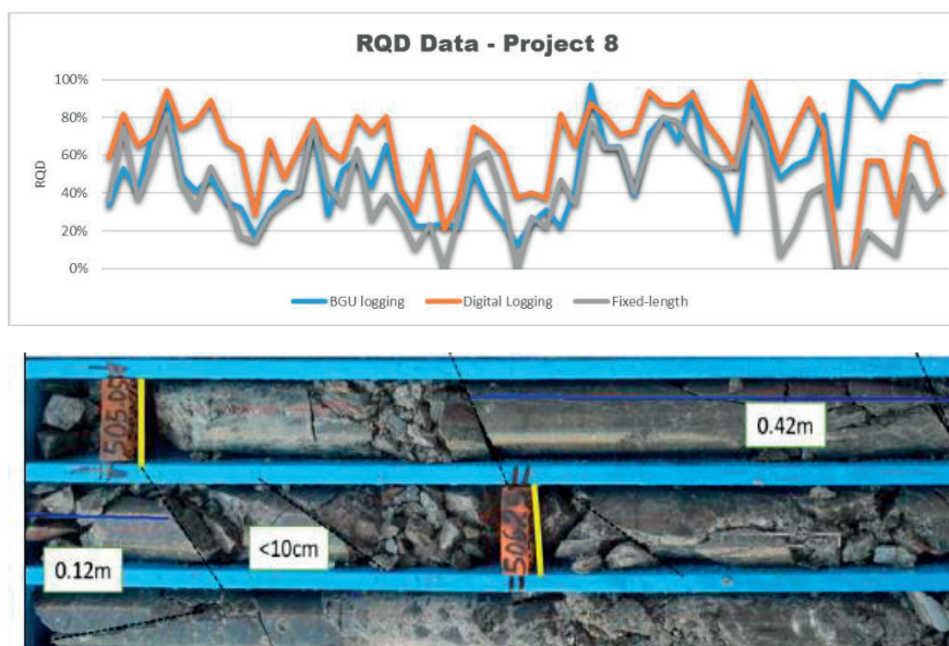
Figure 2 Example of RQD being underestimated on-site and adjusted during digital logging.
