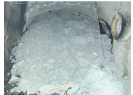
Example of excellent fragmentation at Ridgeway Mine (note: Tyre to be used as a marker for seeding the cave)
