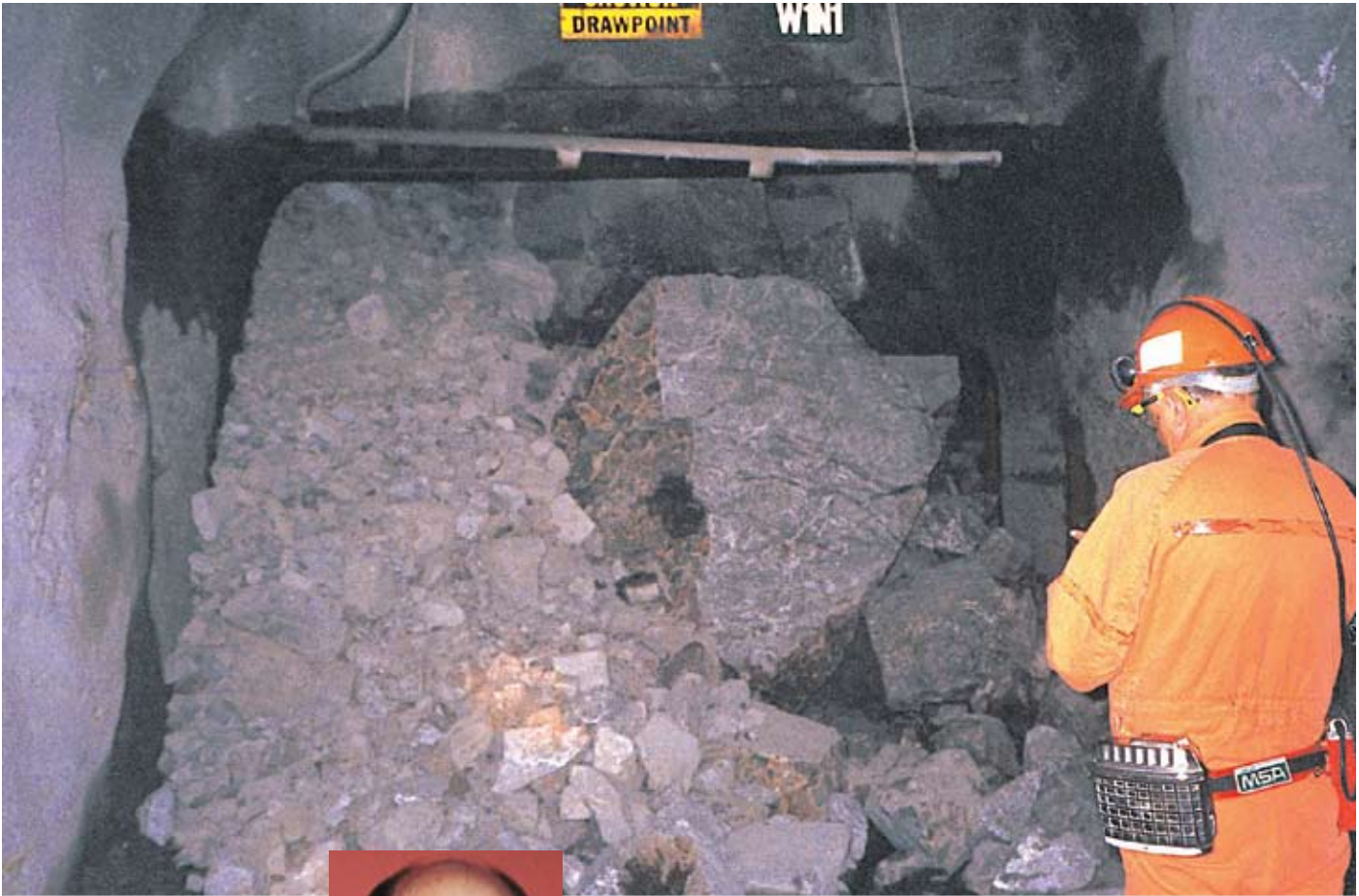
A large rock fragment in a drawpoint at the Northparkes mine, Australia
